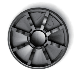
Plastic Support after Hammering (8 supporting block become deformed, and fit with the screw)
