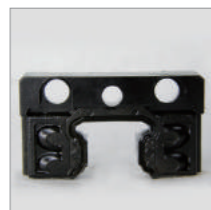
End seal in good condition
